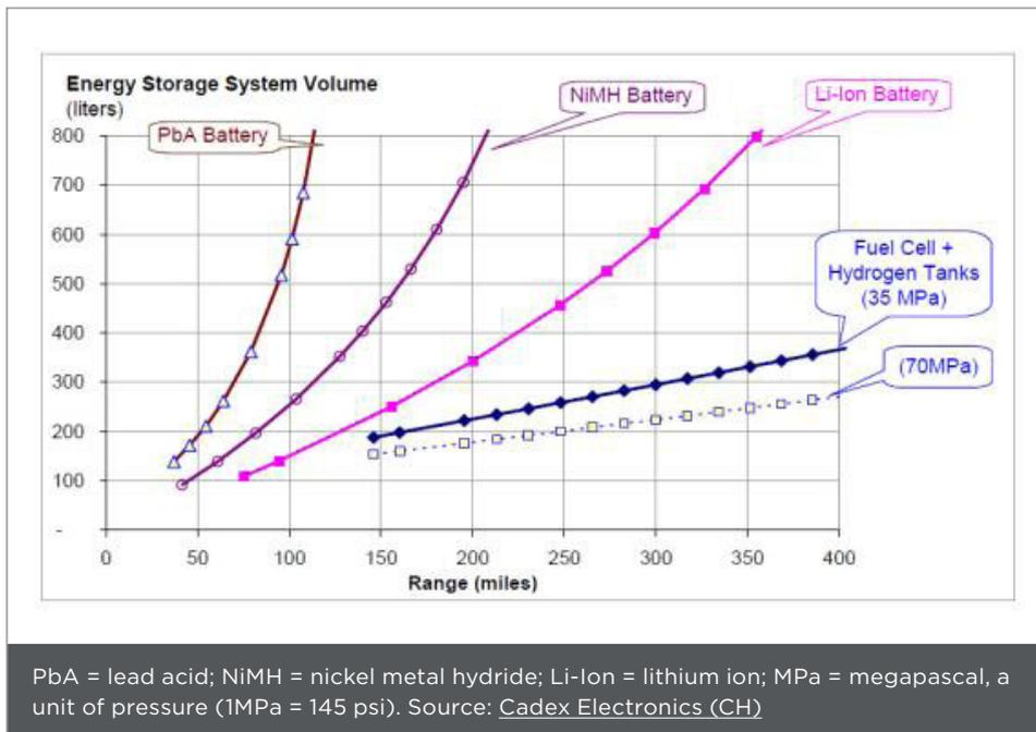
The driving range as a function of energy storage by volume is linear on ICEs and FCEVs, but the driving range of a BEV in terms of energy storage is logarithmic.
